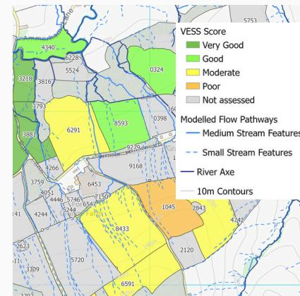
Infiltration is limited across the catchment and therefore the risk of runoff is increased - structure risk assessments are required before spreading manure.
