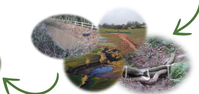
**Transport:** Disrupt transport pathways. Slow & filter runoff. Reduce connectivity.
